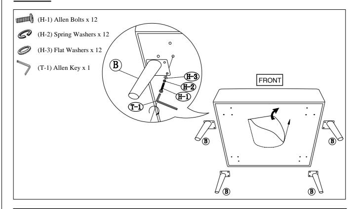
Lay Seat(A) down on its back on a padded,non-marring surface. Open the zipper dust cover and remove the 4 Legs(B) as illustrated. Align the mounting plate holes on each Leg(B) with the corresponding pre-threaded holes at each corner of Seat(A) as shown. Secure each Leg(B) using Allen Bolts(H-1), Spring Washers(H-2) and Flat Washers(H-3), stacking the hardware in the order shown. Engage all bolts by hand, then fully tighten using Allen Wrench(T-1). Close the zipper dust cover when complete.
